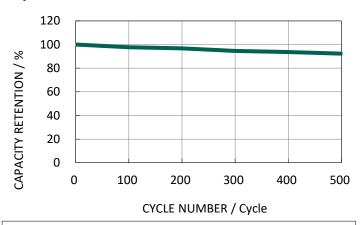
Charging Condition : CV(2.6V, 100 $\Omega$ , 24H, 20°C) Discharging Condition : CR(4.7k $\Omega$ , 2.0V Cut-off, 20°C)
