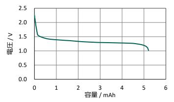
Charging Condition : CV(2.3,  $100\Omega$ , 16H,  $20^{\circ}$ C)
