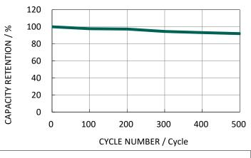
Charging Condition :  $CV(2.6V, 51\Omega, 24H, 20^{\circ}C)$ Discharging Condition :  $CR(2.0k\Omega, 2.0V Cut-off, 20^{\circ}C)$
