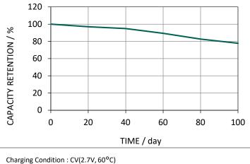
Discharging Condition :  $CR(20k\Omega, 2.0V \text{ Cut-off}, 20^{\circ}\text{C})$
