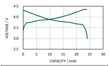
Charge Condition: CC/CV 22.0mA(1C) - 4.35V, 1.1mA(0.05C) cut-off at  $20^{\circ}$ C Discharge Condition: CC, 4.4mA(0.2C) - 3.0V cut-off at  $20^{\circ}$ C
