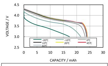
Charge Condition: CC/CV 11.0mA(0.5C) - 4.35V, 1.1mA(0.05C) cut-off at  $20^{\circ}$ C Discharge Condition: CC, 4.4mA(0.2C) - 3.0V cut-off at  $20^{\circ}$ C
