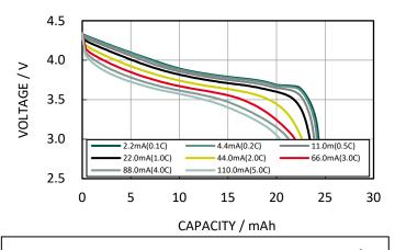
Charge Condition: CC/CV 11.0mA(0.5C) - 4.35V, 1.1mA(0.05C) cut-off at 20°C Discharge Condition: CC, 3.0V cut-off at 20°C
