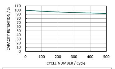
Charge Condition: CC/CV 22.0mA(1C) - 4.35V, 1.1mA(0.05C) cut-off at  $20^{\circ}$ C Discharge Condition: CC, 22.0mA(1C) - 3.0V cut-off at  $20^{\circ}$ C
